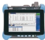
Optical spectrum analyser FTBx-5235
